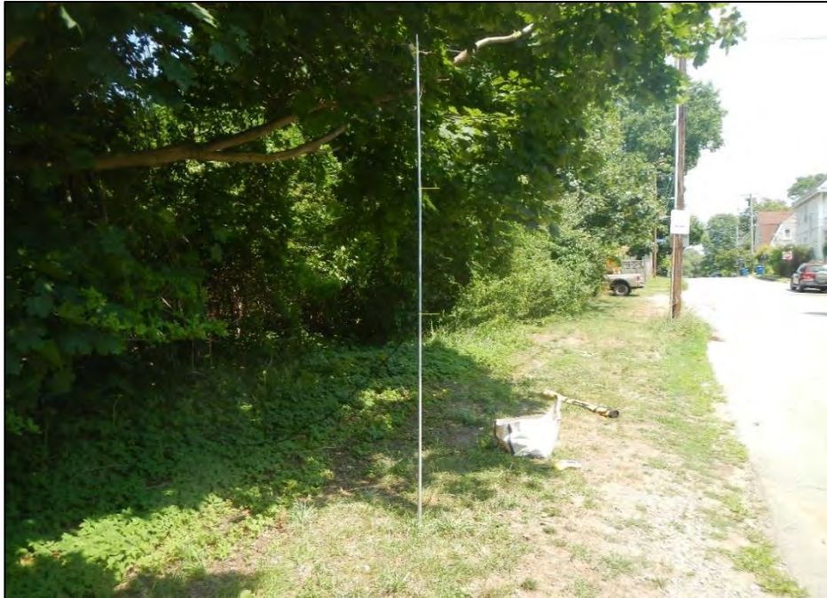
Photo 1: An easterly view of detector # D003 on the northern shoulder of Sycamore Street. The detector was set up for two consecutive survey nights from August 6 to August 8, 2018. The cone of detection was oriented to the west to be parallel to the traffic flow and minimize extraneous noise from passing vehicles.
