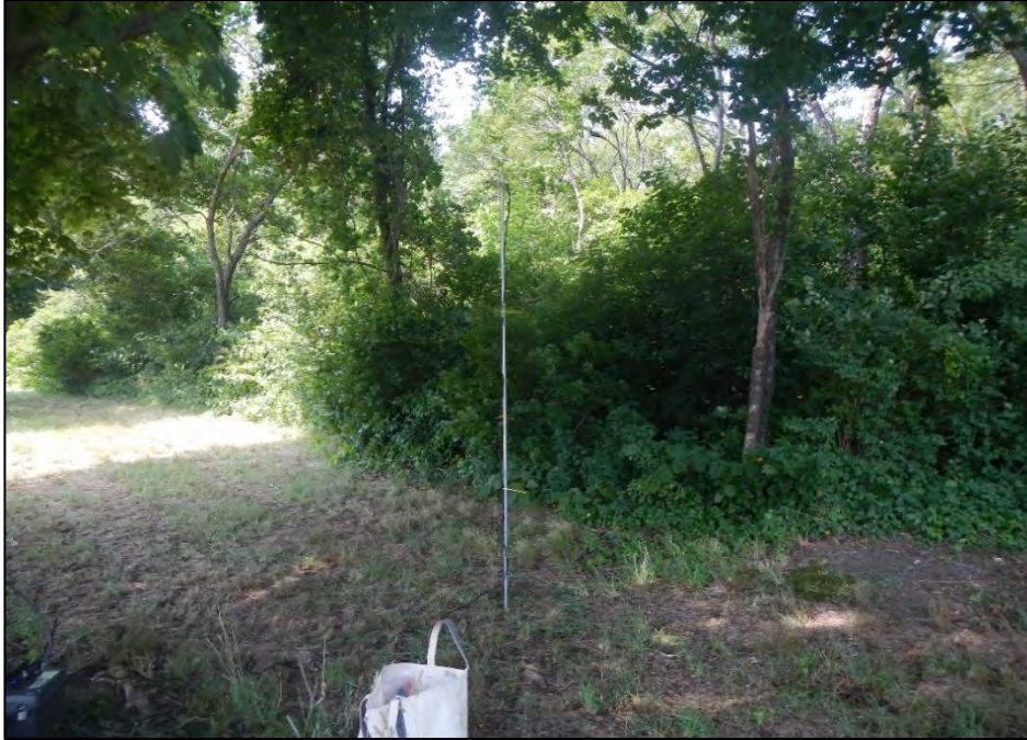
Photo 5: A northeasterly view of detector # D005 on the eastern shoulder of Girard Avenue adjacent to Miantonomi Park. The detector was set up for two consecutive surveys nights from August 6 to August 8, 2018. The cone of detection was oriented to the north to be parallel to the traffic flow and minimize extraneous noise from passing vehicles.
