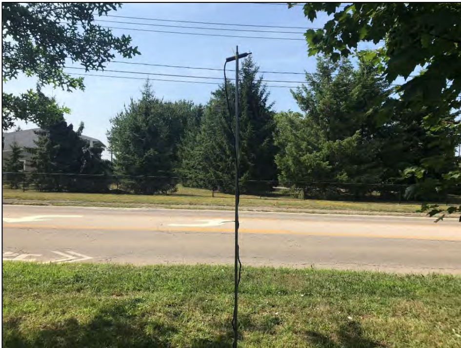
Photo 8: A view looking west towards the detector. The detector was set up approximately 10-feet from the road edge.
