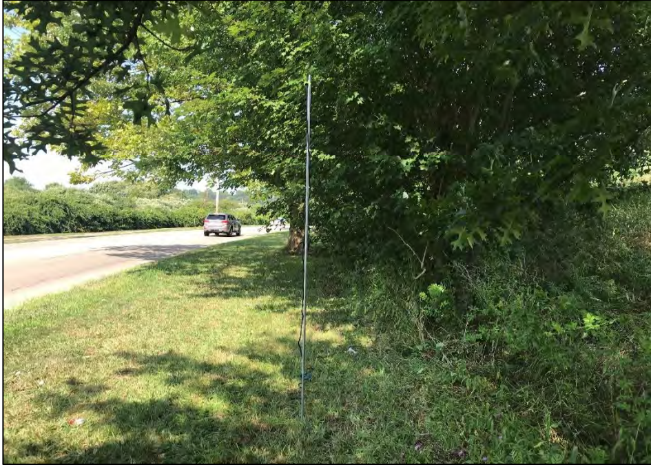
Photo 7: A northeasterly view of detector # D006 on the eastern shoulder of Coddington Highway. The detector was set up for two consecutive surveys nights from August 6 to August 8, 2018. The cone of detection was oriented to the northeast to be parallel to the traffic flow and minimize extraneous noise from passing vehicles
