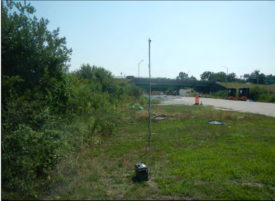
Photo 3: A southerly view of detector # D004 setup on the highway infield between Route 238 and an abandoned ramp. The detector was set up for two consecutive surveys nights from August 6 to August 8, 2018. The cone of detection was oriented to the south to be parallel to the traffic flow and minimize extraneous noise from passing vehicles.
